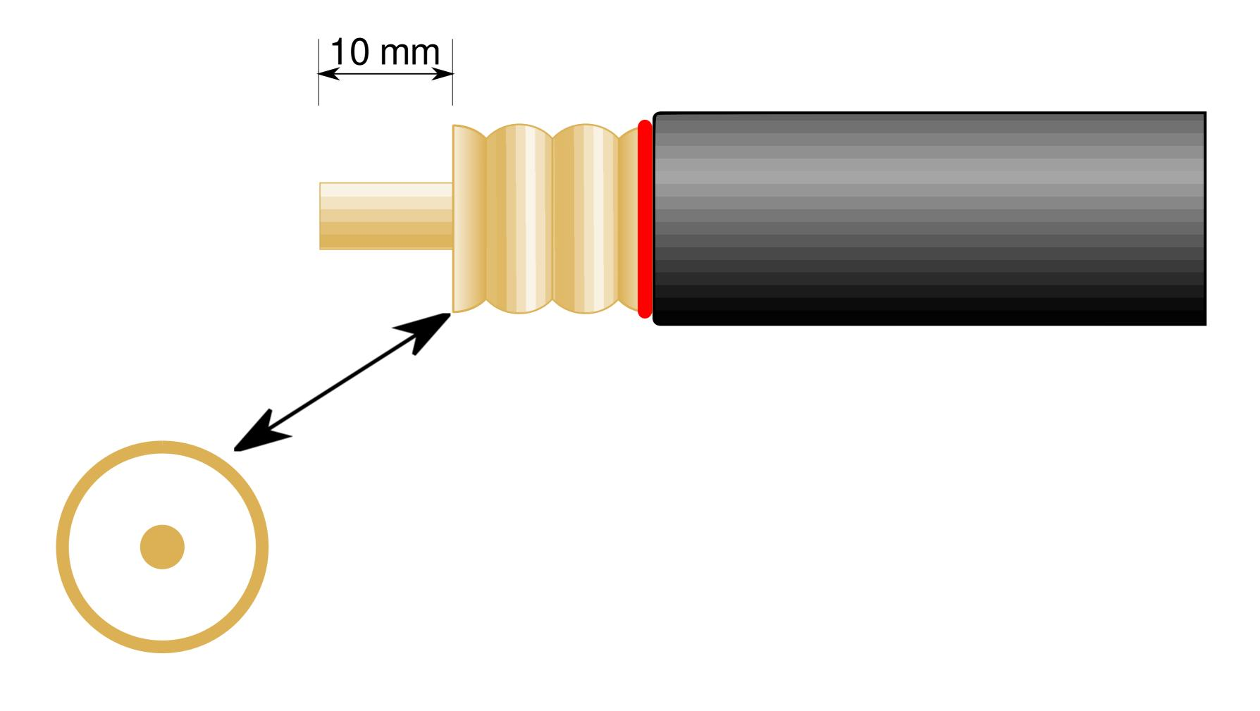
Cut the centre condutor so that 10mm is protruding from the dielectric. Ensure the end of the centre conductor is flat and clean of and debris or dielectric material
