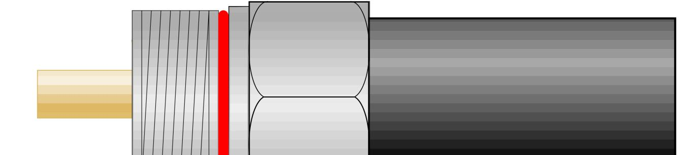
With two spanners, hold the locking nut stationary and tighten the connector body onto the locking nut
